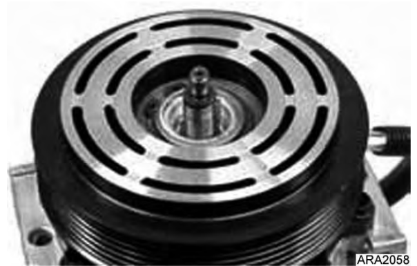
Figure 66: Armature Plate Installation
