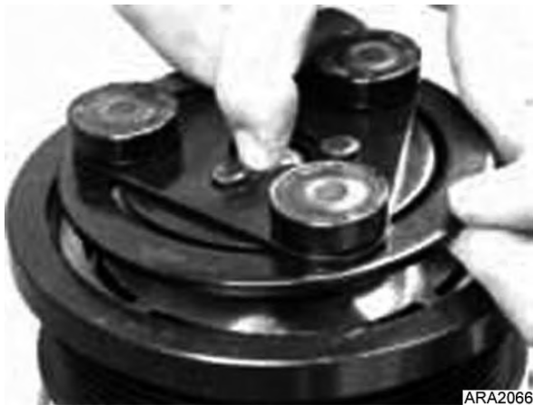
Figure 69: Place Armature on Top of Shaft
