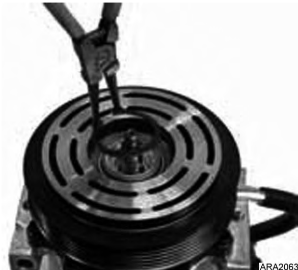
Figure 65: Install Snap Ring
