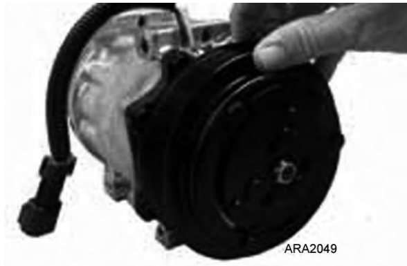
Figure 43: Pulley or Rotor Spin Check
