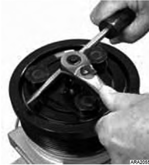
Figure 56: Armature Nut Removal – Swash Compressor
