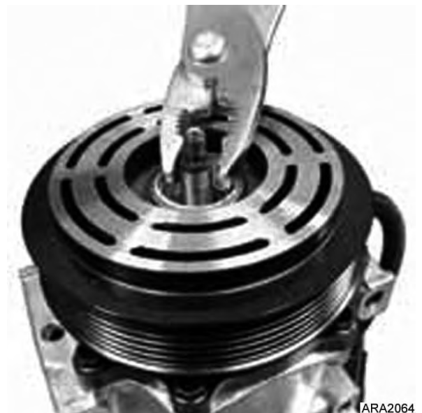
Figure 67: Install Shaft Key
