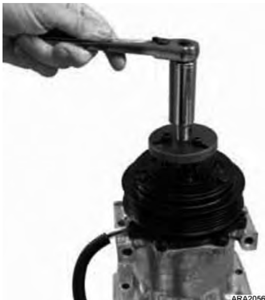
Figure 57: Armature Removal – Wobble Type
