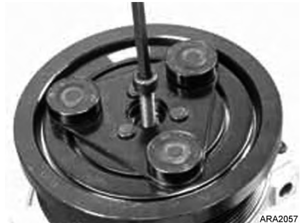
Figure 58: Armature-Removal – Swash Type
