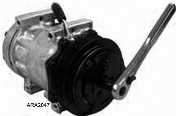
Figure 40: Compressor Rotation Test
