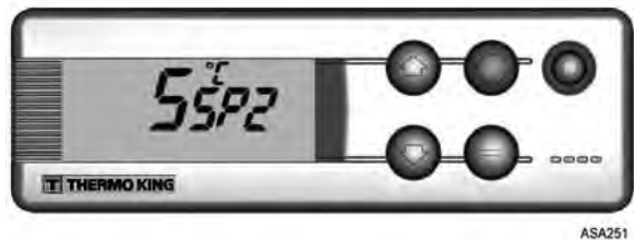
Figure 18: Remote Compartment Setpoint
