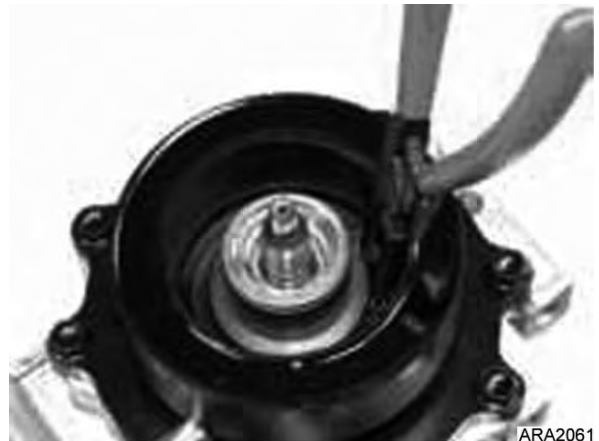
Figure 62: Remove Snap Ring
