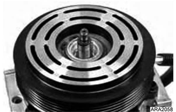
Figure 59: Remove Clutch Accessories
