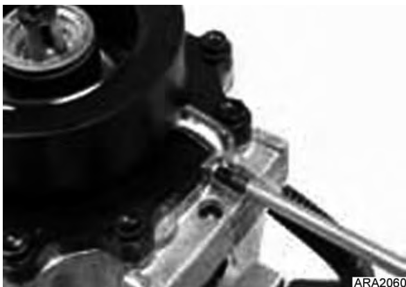
Figure 61: Loosen Lead Wire Clamp Screw
