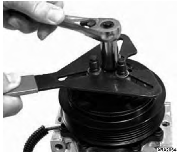
Figure 70: Tighten Armature Nut – Wobble Compressor
