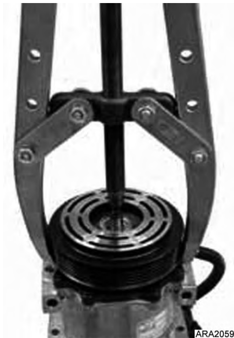
Figure 60: Clutch Pulley Removal
