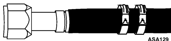
Figure 35: Manually Inserting Fitting
