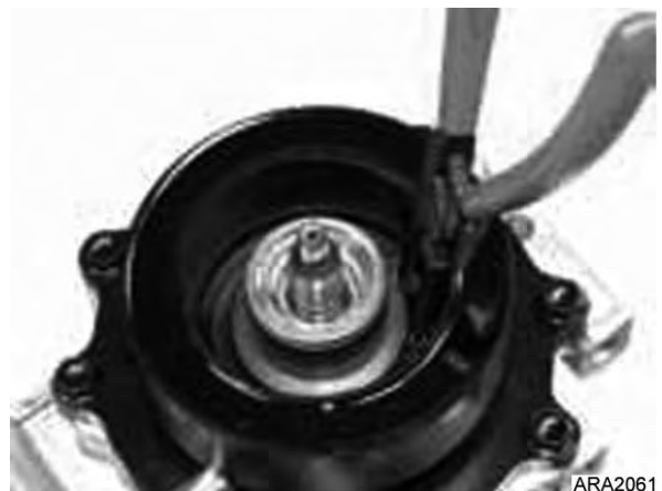
Figure 63: Install Snap Ring
