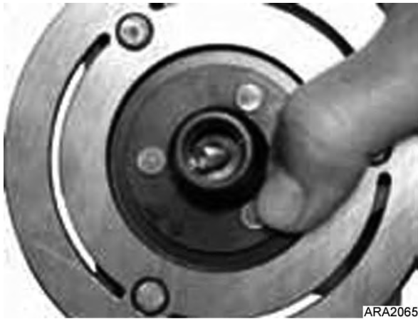
Figure 68: Insert Armature Nut Into Hub
