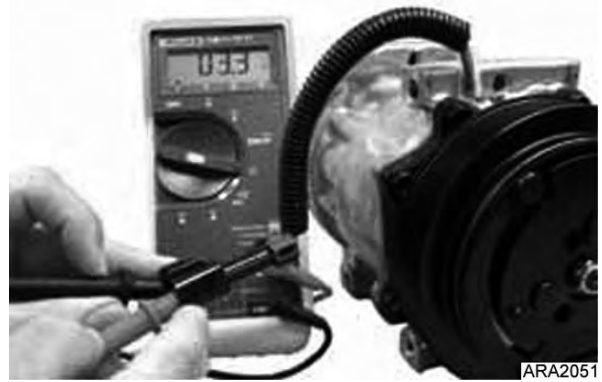
Figure 45: Coil Resistance Check
