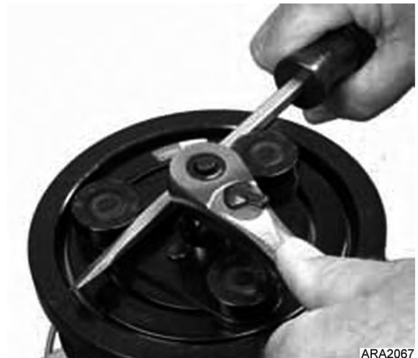
Figure 71: Tighten Armature Nut – Swash Compressor
