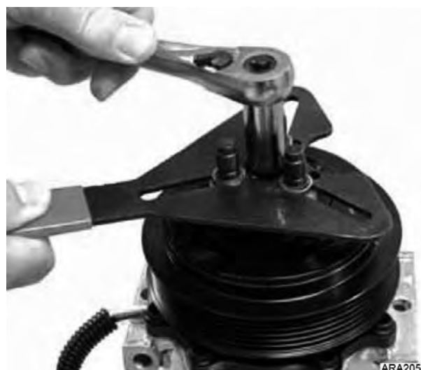
Figure 55: Armature Nut Removal – Wobble Compressor
