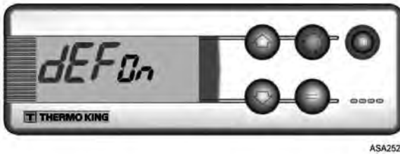
Figure 20: Defrost Condition On
