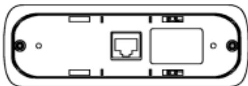
**In-Cab Controller Keypad/Display Unit Rear View**
