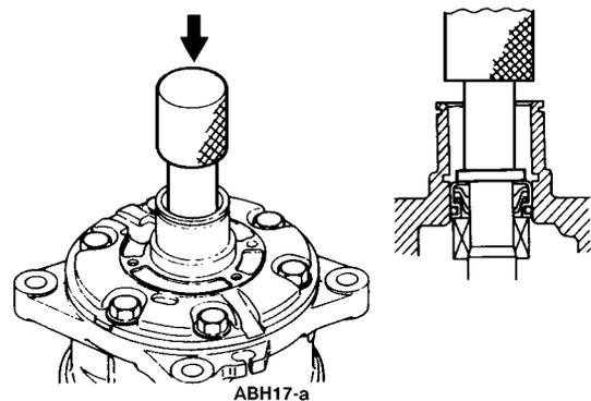
**Press Seal Into Cylinder Head**
