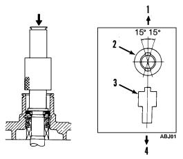
Figure 57: Proper Shaft Seal Cover Position
