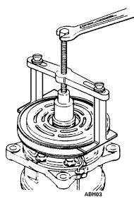
Figure 43: Remove Pulley
