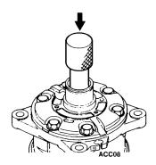
Figure 56: Install Shaft Seal Cover
