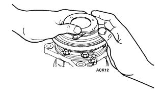
Figure 41: Remove Drive Plate
