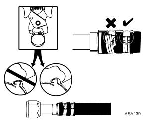
Figure 37: Tightening Both Clips
