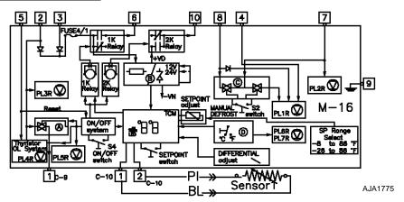
Figure 19: BLOCK DIAGRAM M-13, M-16
