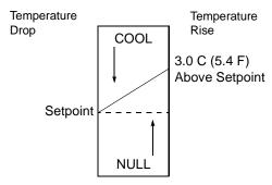
Figure 4: Thermostat Algorithm
