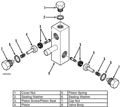
Figure 28: Check Valve Assembly
