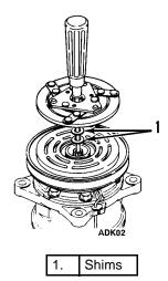
Figure 49: Install Shims and Drive Plate
