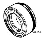
Figure 52: Inspect Shaft Seal
