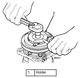
Figure 40: Remove Center Bolt
