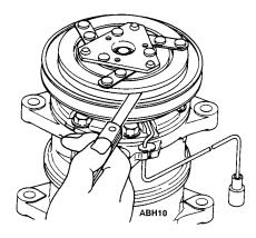
8. Ensure that the clutch clearance is as specified. If necessary, adjust the clearance using shims.
