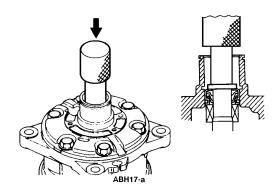
Figure 55: Press Seal Into Cylinder Head
