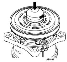
Figure 47: Install Pulley
