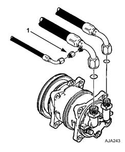
1. Liquid Injection Metering Orifice
