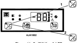
Figure 11: On/Off Key & LED
