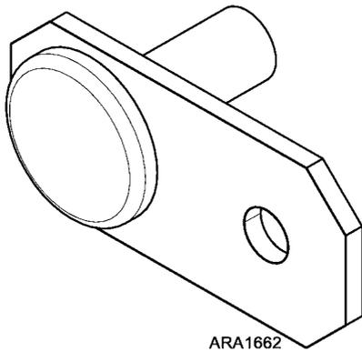
Figure 230: Close Up of Blade Pivot
