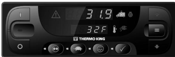
Figure 10: SR-2 Truck HMI Controller
