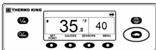
Figure 74: High Speed Lockout Key
