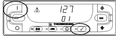
Figure 31: ON and PRETRIP TEST Keys
