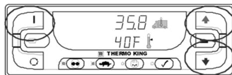
Figure 37: ON Key, UP/DOWN Arrow Keys
