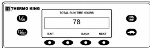
Figure 105: Scroll Through Hourmeters
