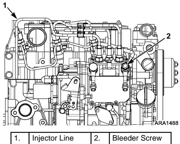
**Figure 169: Injection Pump**
