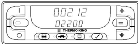
**Figure 39: Software Revision and Serial Number**
