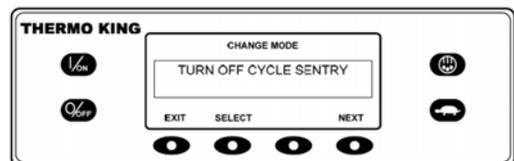
Figure 111: Turn Off/Turn On CYCLE-SENTRY Screen
