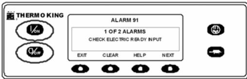
Figure 68: Prompt Screen, standby power is turned off or is no longer available
