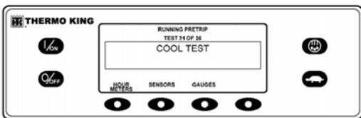
Figure 133: Performing Cool Test
