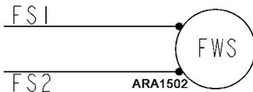
Figure 150: Flywheel (RPM) Sensor Wires
