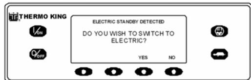
Figure 135: Standby Power connected & available
