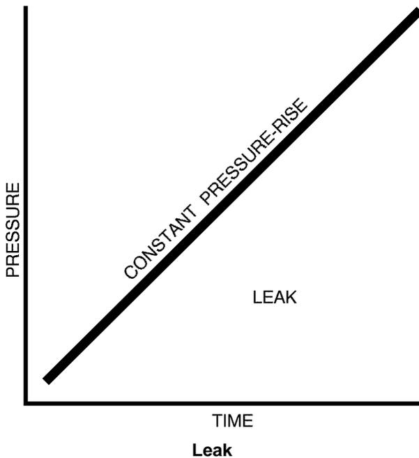
Isolate the pump from the system by closing the proper valve. Watch the movement of the vacuum gauge needle. If the needle continues to rise, this is an indication that a leak exists in the unit or the connecting line. The leak must then be located and eliminated.
