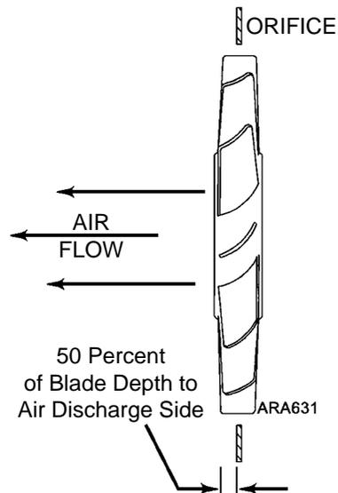
Figure 227: Fan Blade Position in Orifice for Ten-Blade Fan
