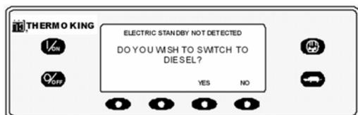
Figure 138: Prompt for Switch to Diesel
