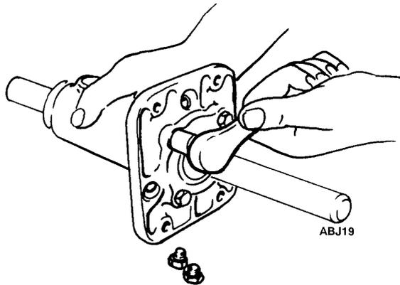
**Figure 233: Removing Bearing Retainer Bolts**
