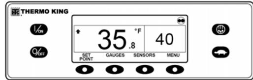
Figure 65: Standard Display of Temperature and Setpoint
