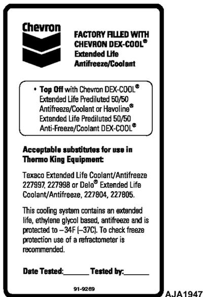
**Figure 163: ELC Nameplate Located On Expansion Tank**
