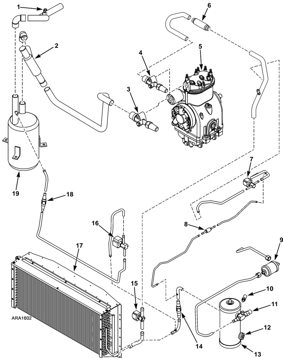
**Figure 208: Condenser Refrigeration Component Locations in Units with Tube and Fin Condenser Coils (Ending 06/12) (Two-Cylinder Compressor Shown, Similar with Four-Cylinder Compressor)**
