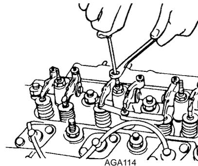
**Figure 187: Adjusting Valves**
