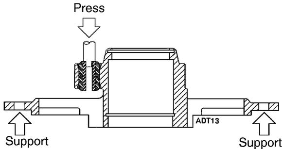
**Figure 221: Bushing Removal**
