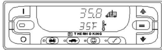
Figure 15: Standard Display of Box temperature and Setpoint
