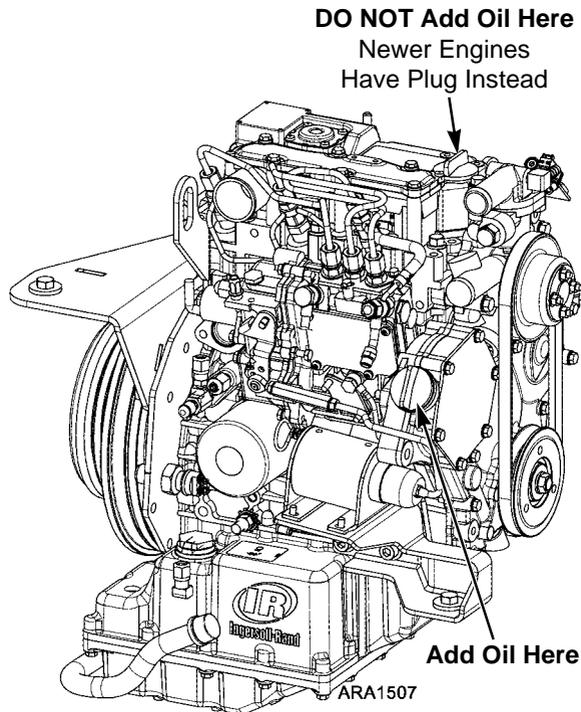
**Figure 157: Oil Cap Locations on Engine**
