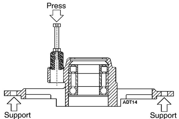
**Figure 222: Bushing Insertion**
