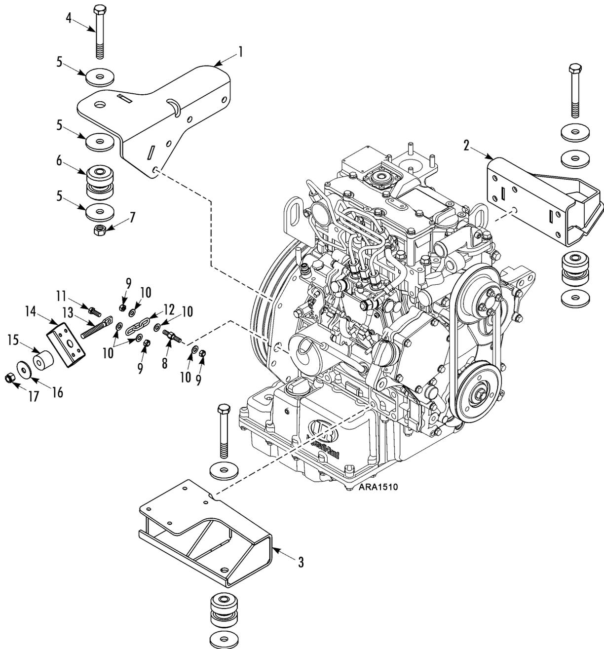
Figure 188: Engine Mounting Components
