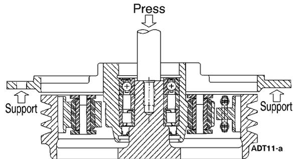
**Figure 219: Housing Removal**
