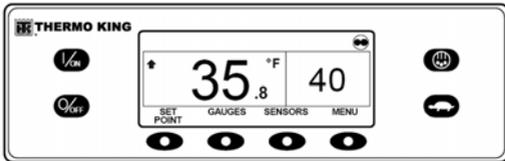
Figure 63: Standard Display of Temperature and Setpoint
