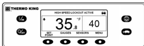
Figure 77: Standard Display, High Speed Lockout Active
