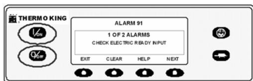
Figure 137: Display when Standby Power not available
