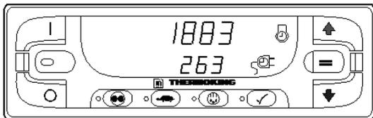
Figure 14: Electric Motor Run Time Hours and Electric Icon
