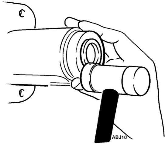
Figure 239: Installing Oil Seal
