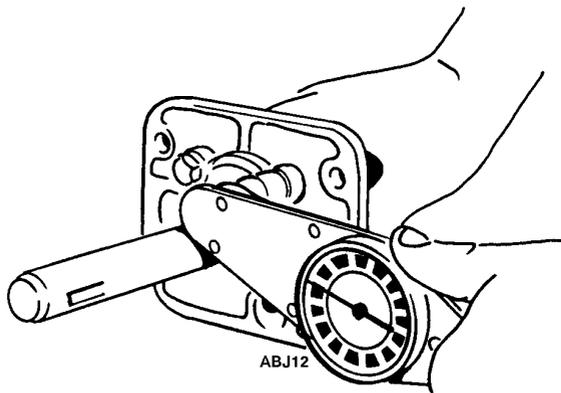
**Figure 241: Torquing Retainer Plate Bolts**
