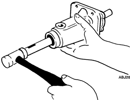
**Figure 234: Removing Shaft**
