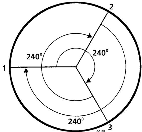
Figure 184: Valve Adjustment and Firing Order
