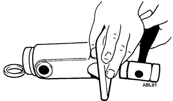
**Figure 235: Removing Oil Seal**
