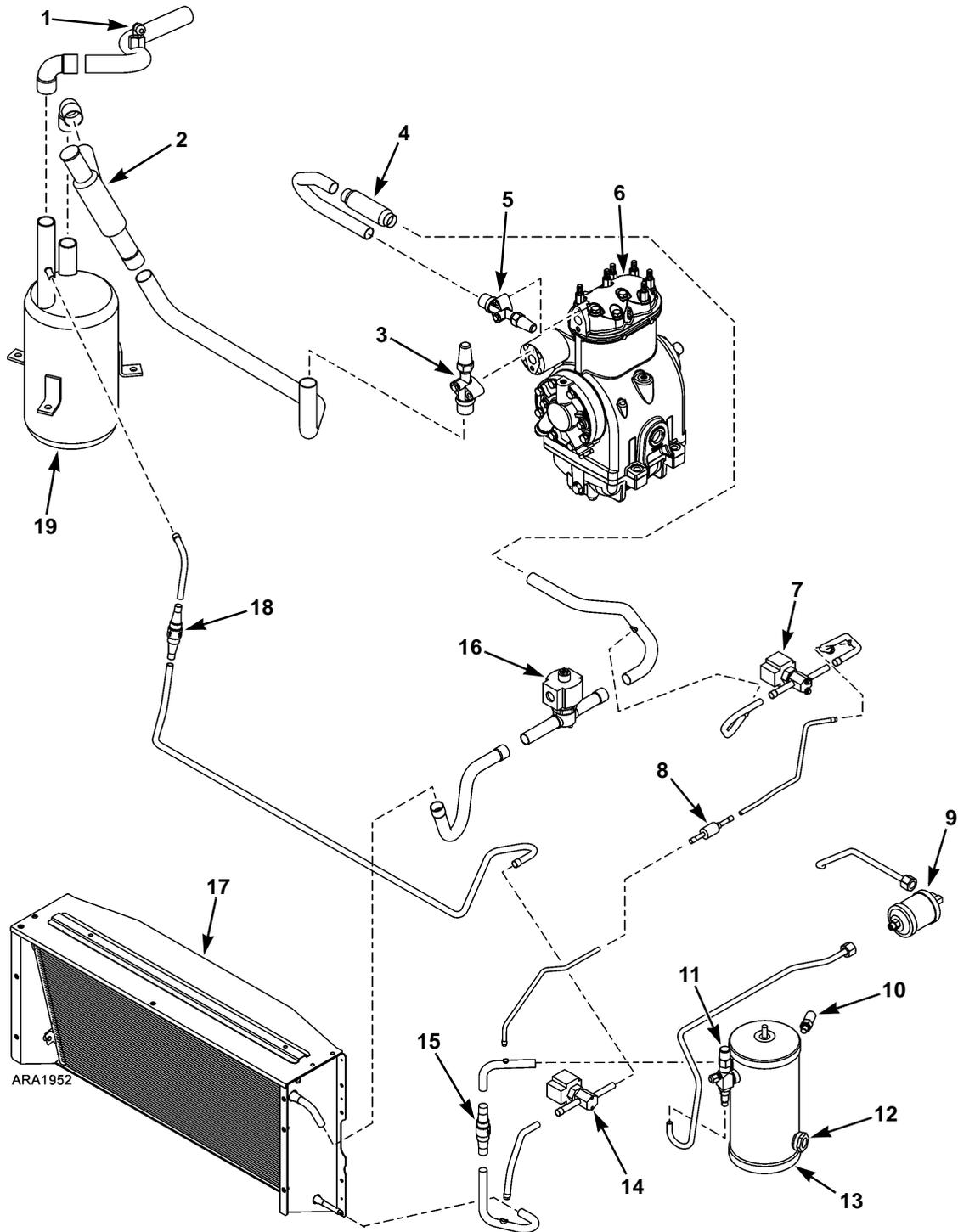
**Figure 209: Condenser Refrigeration Component Locations in Units with Micro-Channel Condenser Coils (Starting 06/12) (Two-Cylinder Compressor Shown, Similar with Four-Cylinder Compressor)**
