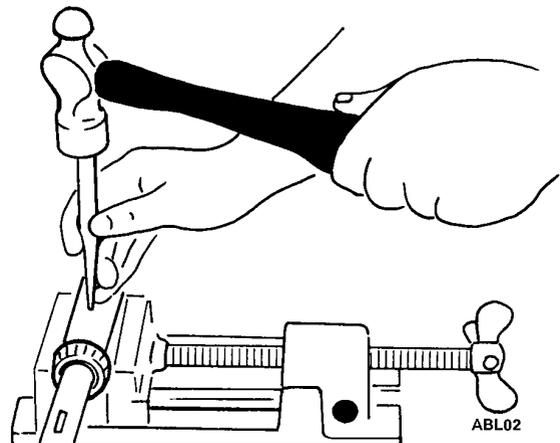
**Figure 236: Removing Roll Pin**
