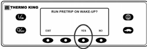
Figure 126: Press Yes Key for Pretrip Test
