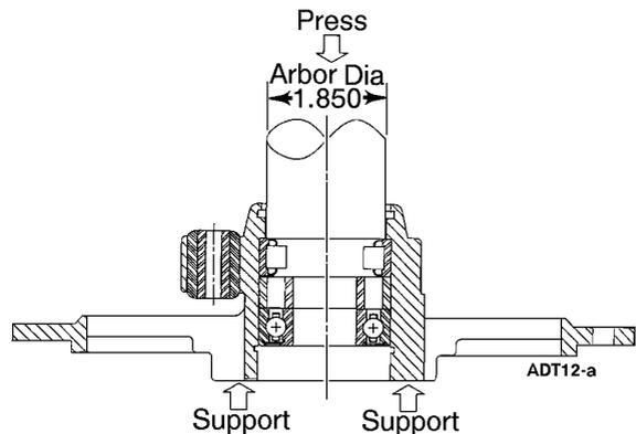
**Figure 220: Bearing Removal**
