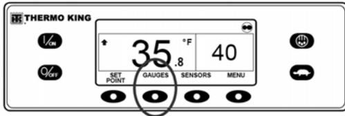
Figure 78: Gauges Key
