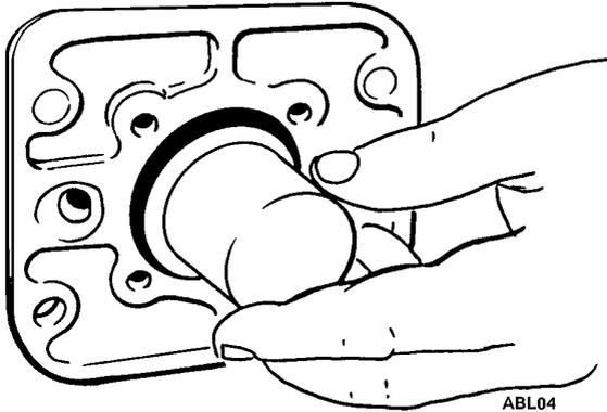
Figure 238: Installing Splash Guard
