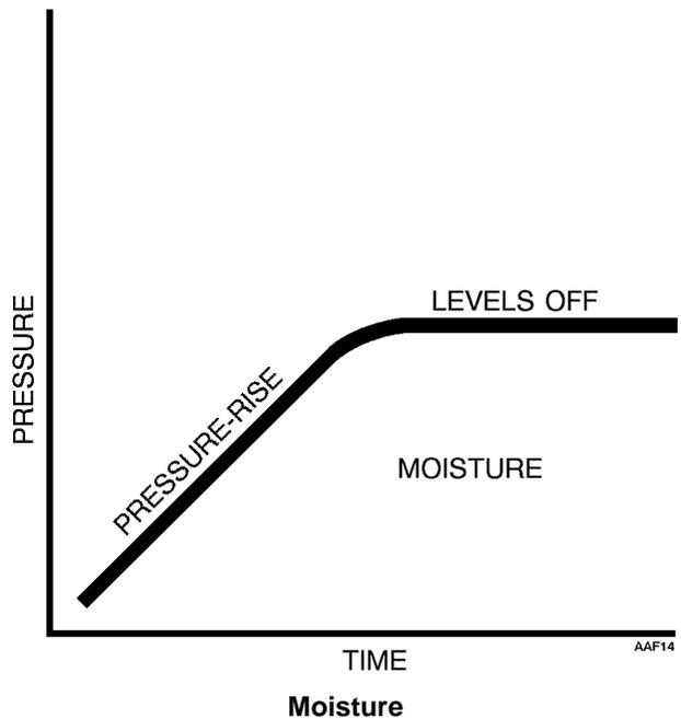
Should the needle show a pressure rise but finally level off to practically a constant mark, this is an indication that the system is vacuum tight but is still too wet, requiring additional dehydration and pumping time.
