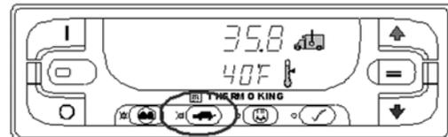
Figure 27: HIGH SPEED LOCKOUT Key
