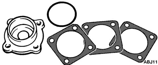
Figure 240: Shims and O-ring
